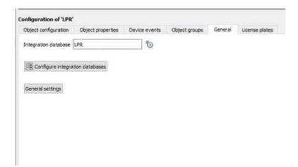
Currently the general tab deals with the **Integration database**. Here, select an existing database, or configure a new database for the integration.
