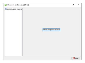
The first time an integration database is added, initialise this feature on the unit. This will add a broad database, within which all of the integrated device's databases will be added.
