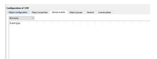
This lists all Events sent from the device. It is an excellent way for installers to see that the integration is functioning, and to monitor the Events happening on site.
