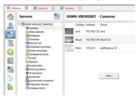
The Axis camera's driver, and IP address are listed below:
